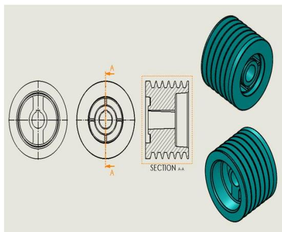
**Fig 3.1.**Pulley Model Drawings.
