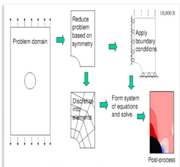
Fig.2.1. Finite Element Procedure
