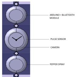
Figure 1: Pictorial representation of the watch in CAD
