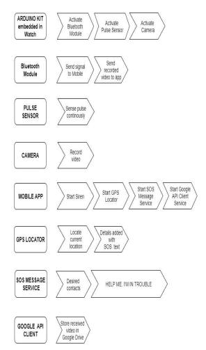
Figure 2: Schematic representation of the components with their functions
