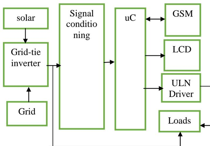
Fig.3. Architecture of Hybrid Solar System
