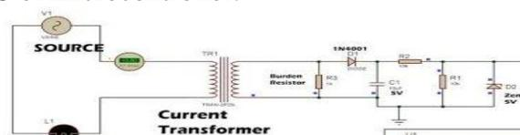
Fig. 4 current transformer
