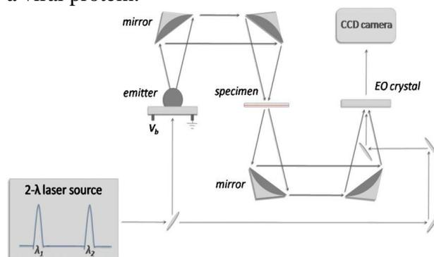
Fig.2: The 2D THz Imaging System
