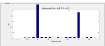
Fig. 13.THD analysis of Inverter with AC voltage regulator at its load
