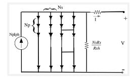
Fig. 3. Equivalent model of PV array
