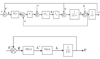
Fig. 7. Block diagram of outer loop
