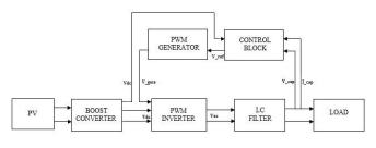
Fig. 1. Block diagram of Grid connected PV system
