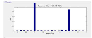
Fig.11. THD analysis of Inverter with uncontrolled rectifier as load
