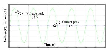
Fig. 12. Simulation output with non linear load – Ac voltage controller.
