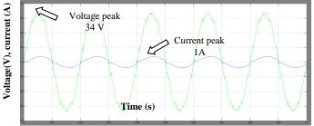
Fig. 10. Simulation output with non linear load -Uncontrolled rectifier.
