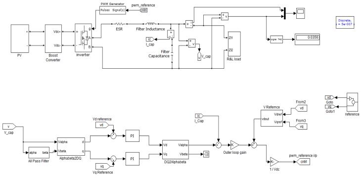
Fig. 4 – Simulation model of the inverter control.
