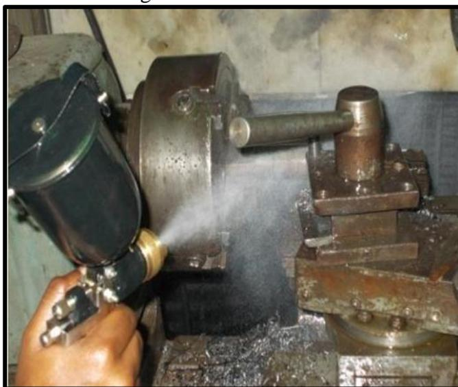
Fig. 5: A view of turning by synthetic oil
