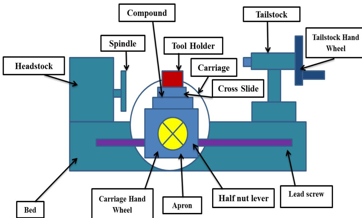
Fig. 1: A view of Lathe Machine diagram
