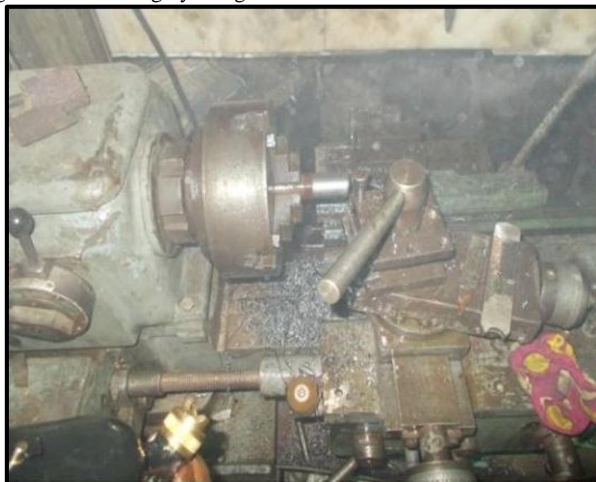
Fig. 4: Aview of turning by using natural oil
