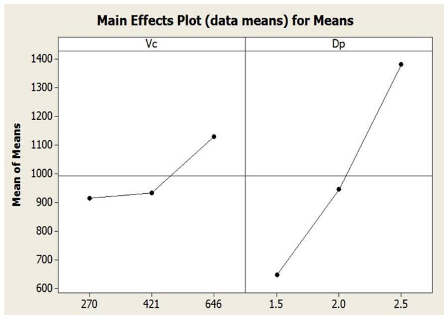
Figure 6: Shows Graph b/w V<sub>c</sub>, D<sub>p</sub> to MRR
