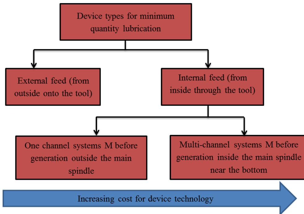
Fig.3: Flow chart of devices types of minimum quantity lubricant system
