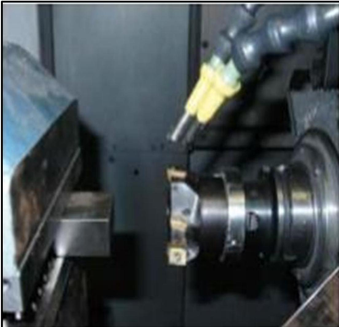
Fig. 2: A view of external feed via nozzles
