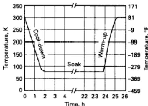
Fig. 2 Plot of temperature versus time for the cryogenic process. Soaking temperature is  $-196^{\circ}\text{C}$  (P.I.Patil & Dr.Bimlesh kumar, 2013)
