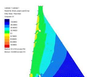
Fig.15 Stresses in Y- direction
