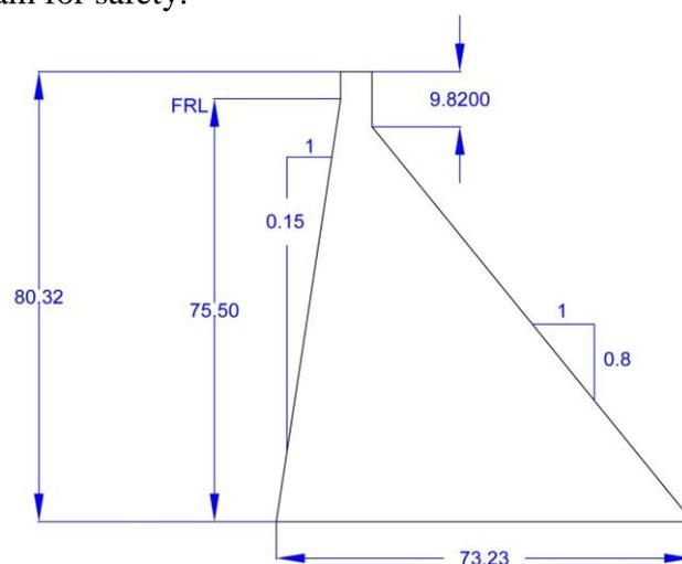
Fig.1 Section of the dam
