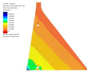
Fig.9 Stresses in Y- direction
