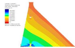
Fig.3 Stresses in Y-direction
