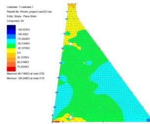
Fig.14 Stresses in X- direction
