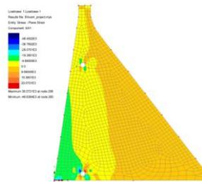
Fig.4 Shear Stresses
