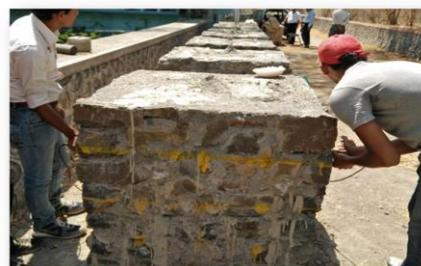
*Step II: Grouting of the dam prototypes using two different grout mixtures:* After the analysis was done for the distressed gravity dam then suitable blocks of sizes 1Mx1Mx1M were prepared using stone masonry which had voids and seepage which resembled the condition of distressed gravity dam. NDT tests were performed on the blocks. The ultrasonic pulse velocity meter was used and the readings were noted as under :
