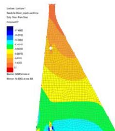
Fig.12 Stresses in Y- direction
