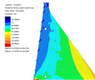
Fig.16 Shear Stresses
