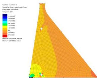
Fig.10 Shear Stresses
