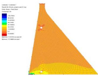
Fig.8 Stresses in X- direction
