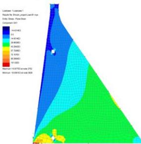
Fig.7 Shear Stresses
