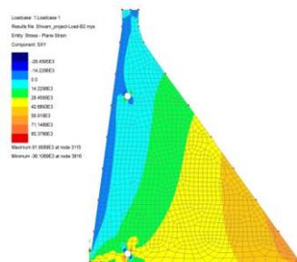
Fig.13 Shear Stresses
