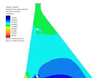
Fig.6 Stresses in Y-direction
