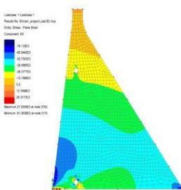
Fig.11 Stresses in X- direction
