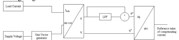
Fig 6. Shunt Active Power Filter
