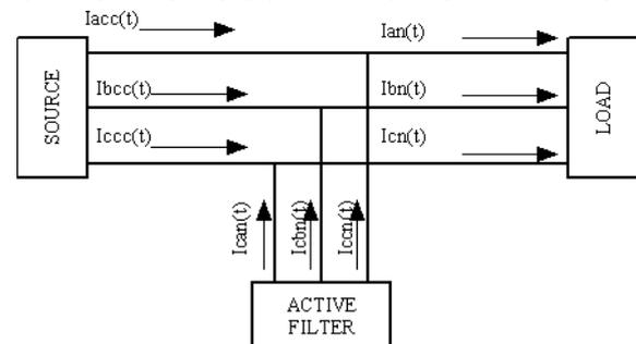
Fig 5. Shunt Active Power Filter
