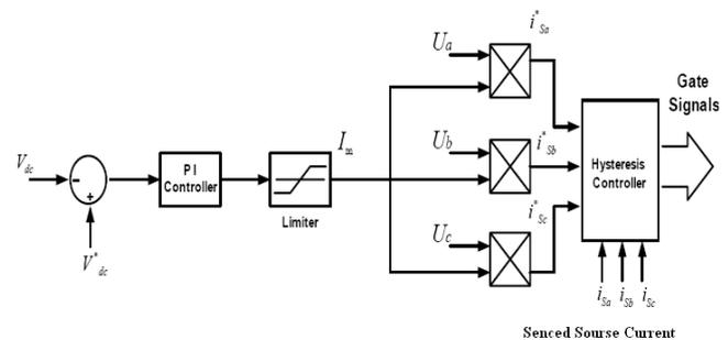
Fig 2 Control block diagram of Unit Vector Template Generation Method
