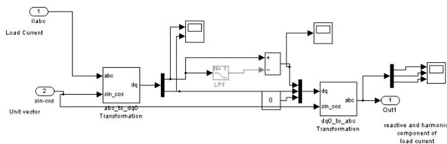
Fig 9. Control block of SRF method
