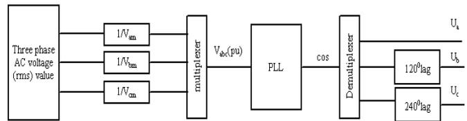
Figure 4 Unit vector template generation using PLL
