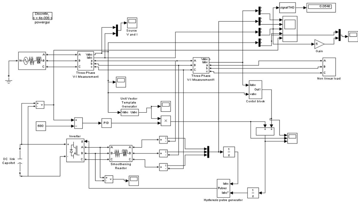
Fig 7. Simulink model of an AHF
