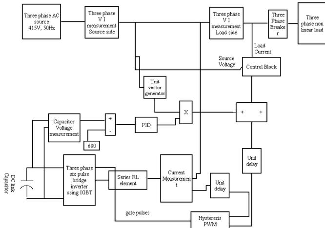
Figure 3 Block diagram representation of AHF
