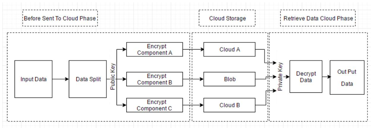
Fig. 2 Workflow structure of splitting data packets in the Distributed data & Storage Process
