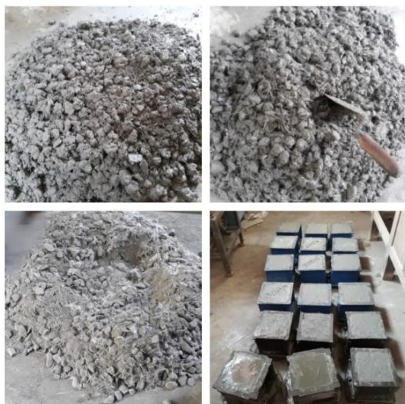
Fig 1: Mixing and moulding of concrete with various fibres and admixtures
