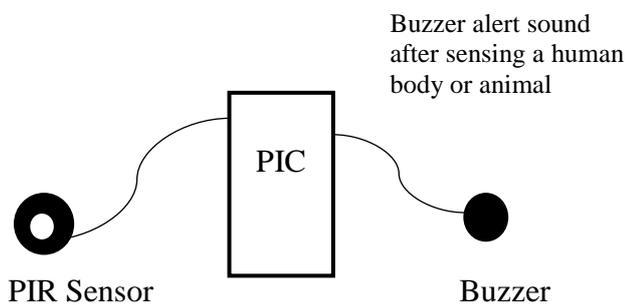
This module works for detecting the human body or animal through the heat as PIR sensors are capable of that, which helps the driver to know about the things moving around the vehicle. [6]
