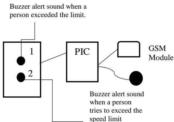
In this module, it consists of two switches. First switch is for speed limit alert; whenever the driver tries to exceed the limit, switch will send the signal
