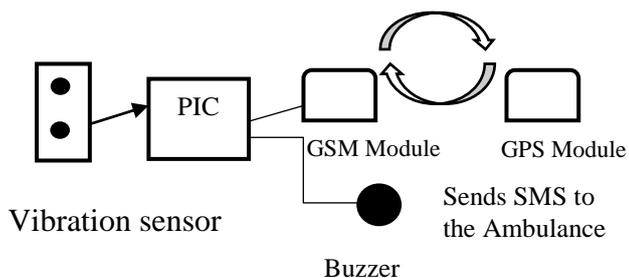
Vibration sensor is the main module of the system. It is used to measure and analyse the velocity or acceleration. In real time, when two vehicles collide with each other and if the frequency exceeds the threshold value then it will send the location of the vehicle where that accident happened. This works with the help of GSM module (Global System for Mobile Communication) connected with GPS module. [3]
