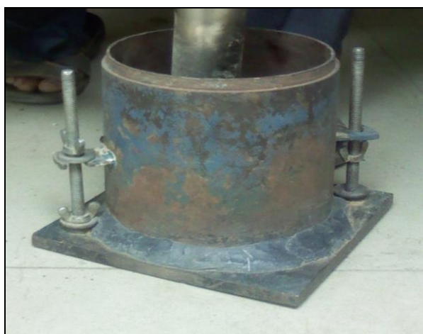
Fig: 7 picture showing the mould used for compacting the aggregates
