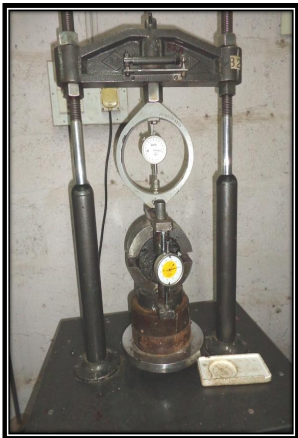
Fig: 12 Specimen being tested in Marshall Apparatus
