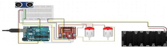
Figure 2: Schematic circuit diagram of the robot
