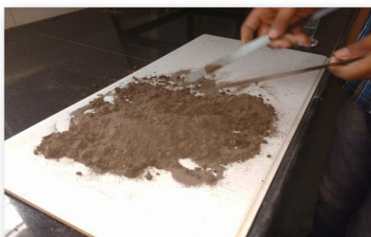
Fig. no.3 dry mixing of RBI GRADE81 in soil
