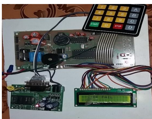
Fig.6 Condition 3: DC fail
