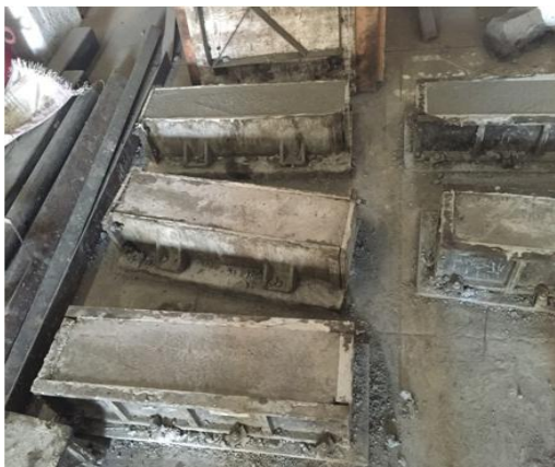
Figure8: - Casting of Cubes
