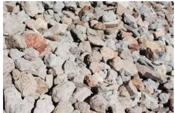
Figure 3: Obtaining Recycled Concrete Aggregates by crushing the Conventional Concrete
