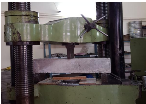
Figure 14: Flexural Test of Concrete
