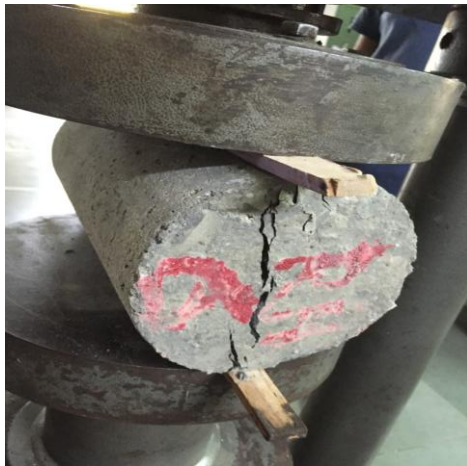
Figure 13: Split Tensile Test of Concrete
