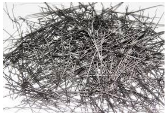
Figure 4: Steel fibers with hooked ends
