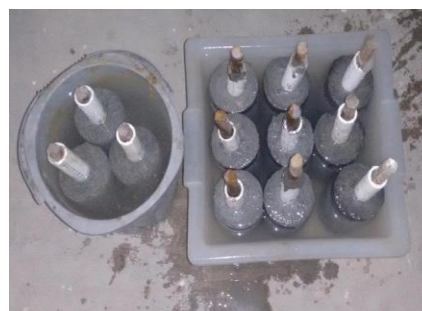
Fig: 2 curing of the Specimens
