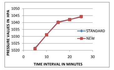
Figure 2: Pressure Sensor Calibration Profile
