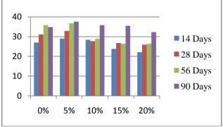
Fig:4 Compressive strength results for Normal concrete and GPP
