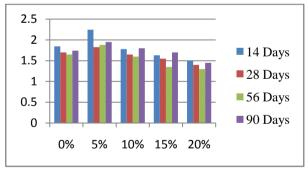
Fig:5 Split tensile strength results for Normal concrete and GPP
