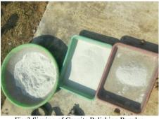
Fig:3 Sieving of Granite Polishing Powder
