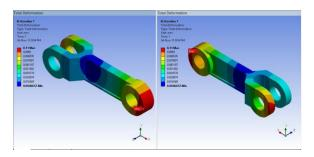
The maximum deformation of the shape of forged chain link is 0.11 mm. The stress and total deformation plots denote that the shape 7 of the link of chain will bear the required load and sustain the stress developed under the given conditions. Thus the optimum shape of the chain has been achieved successfully with considerable amount of material removal from the forged chain link.
