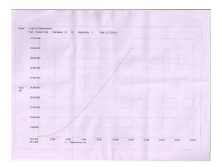
load-displacement plot for optimized cane carrier block conveyor chain which gives us breaking load is 609.65 kN and elongation of 11.8 mm. Here it is observed that breaking happens at fork of the link. Weight
