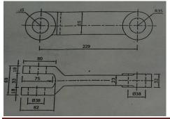
CAD (2D) Model of chain link
