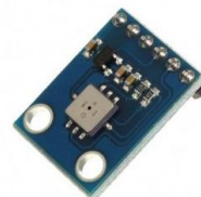
Fig. 4 BMP180 Digital Pressure Sensor
