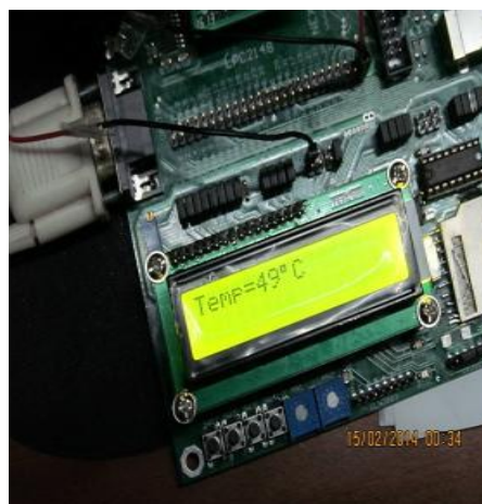
Fig.7. Outputs for LM35 Sensor on LCD
