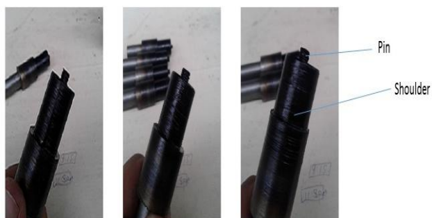
Cylindrical Tool having 18 mm dia
