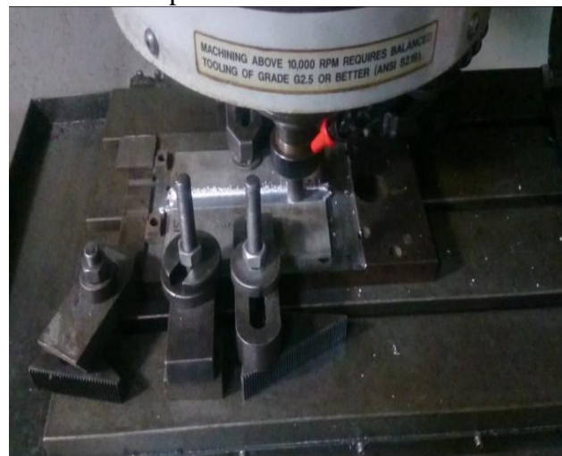
Fig. 3 Work piece set up during FSP
