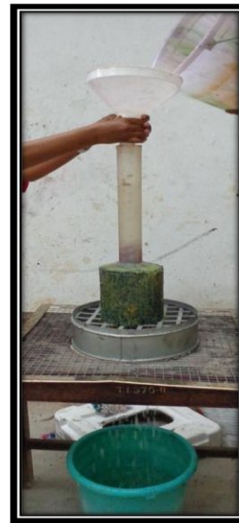
<<< Fig. 6 Pictorial view of compacted specimens used for Moisture Susceptibility test
