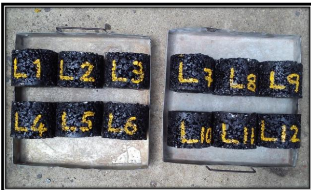
<<< Fig. 6 Pictorial view of compacted specimens used for Moisture Susceptibility test
