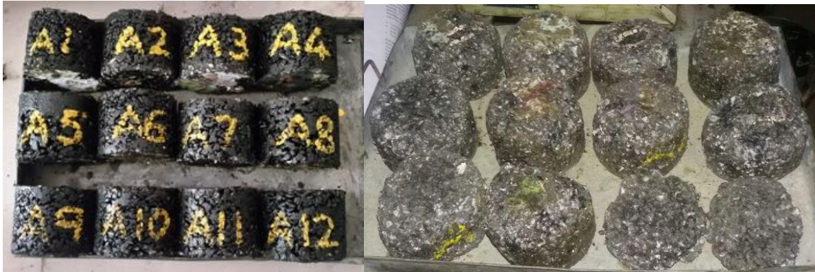
Fig. 2 Compacted aged specimens subjected to test for Ageing Potential
