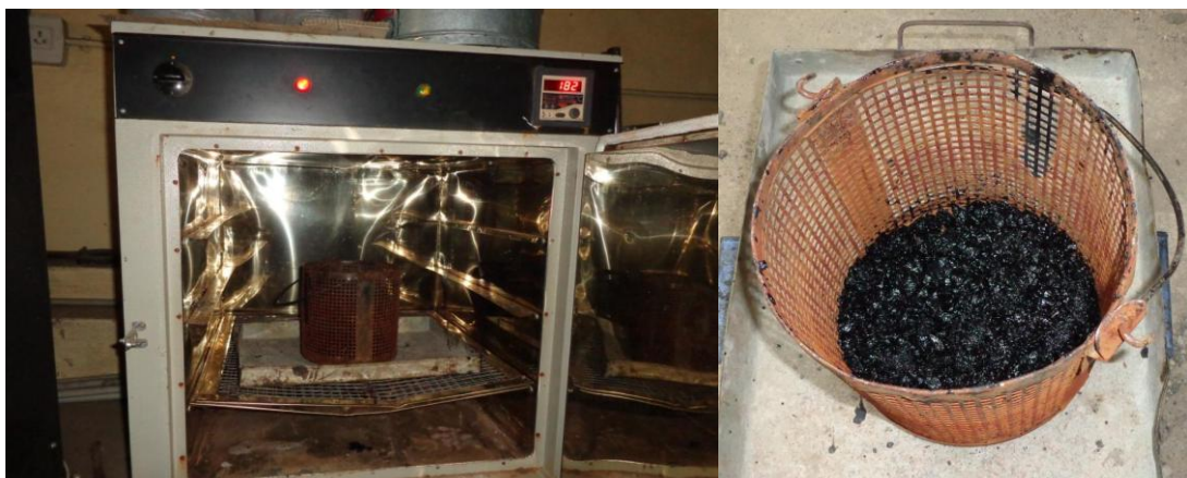
Fig. 3 Un-Compacted specimen subjected to test for Drain-down Potential
