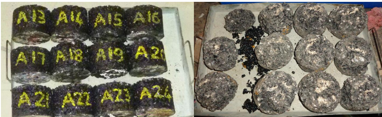
Fig. 3 Un-Compacted specimen subjected to test for Drain-down Potential
