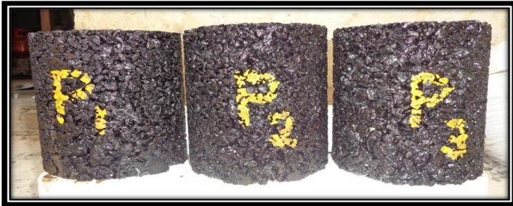
<<< Fig. 4 Pictorial view of compacted specimens for Permeability test (150x150) mm 2
