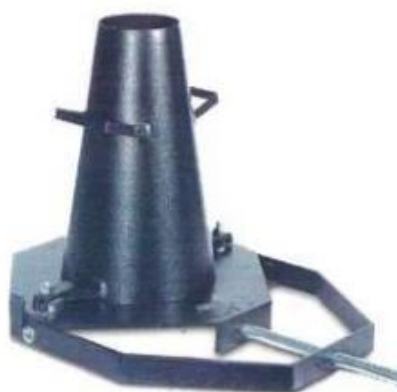
Figure 1: Slump Flow Test Apparatus
