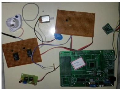
Fig 7: Integration of all sensors with ARM7
