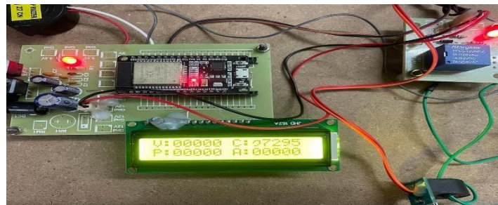
Fig 4.2: LCD parameters display before connecting the load
